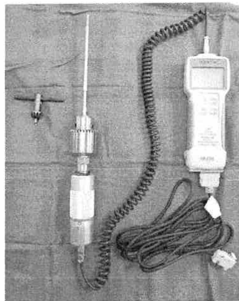
Figure 2. Photograph of a torque measurement device. During the screw insertion, the real-time torque was recorded with a frequency of every 0.05 seconds.
