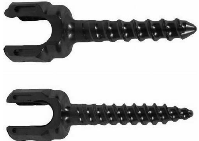
FIG. 1. Details of screws used in this study (length 25 mm, diameter 4.5 mm). Upper: Cancellous screw (Legacy, Medtronic)—outer diameter 4.59 \pm 0.79 mm, root diameter 3.42 \pm 0.46 mm, pitch 2.64 \pm 0.22 mm. Lower: Cortical screw (Solera, Medtronic)—outer diameter 4.54 \pm 0.84 mm, root diameter 3.38 \pm 0.45 mm, pitch 1.99 \pm 0.02 mm.
