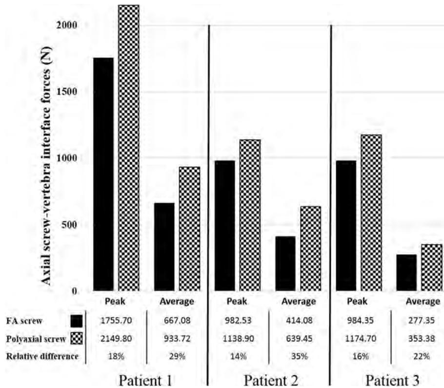
Fig. 5. Peak and average axial screw–vertebra interface forces measured during all steps of the simulated surgery of each patient.
