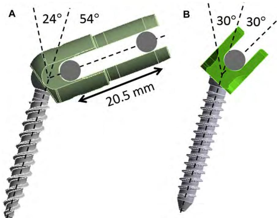
Fig. 2. Differences in screw head pivot and rod capturing distance between (A) favored angle and (B) polyaxial screws as simulated in the model.
